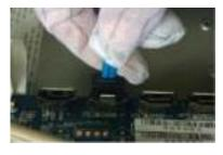
Connect the other end of HDD cable to the mainboard
