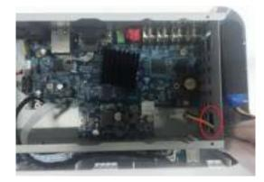
1. Put the battery cable through the hole.
