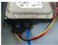
Use the HDD cable and power cable to connect HDD and mainboard.
