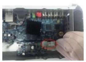
2. Connect to the cable into the port.
