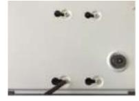
Turn the device to see the back side of it. Aim the screws of the HDD at the holes on the back of the device, and then fix the screws.
