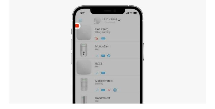
If a hub fault is detected (e.g., no external power supply is available), a faults counter is displayed on the device icon in the Ajax app.
