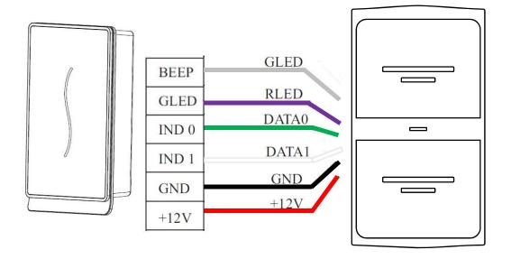
1- Make the connection with the StandAlone equipment in the Wiegand input as shown in the figure.
