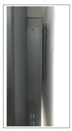
1.2 As you can see in the image, we have on the back of our screen, on the right side we will see a plate with two screws, we just have to remove them to release the OPS module bay
