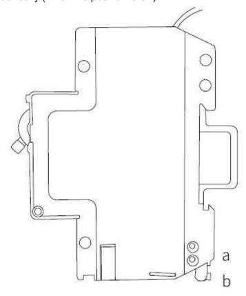
3. Make the connections as shown below: With the switch in the Off position, connect the Line wire to the device terminal (32A), and the Neutral wire to the device Neutral terminal. Connect the distribution board with the screws and close the distribution panel.
