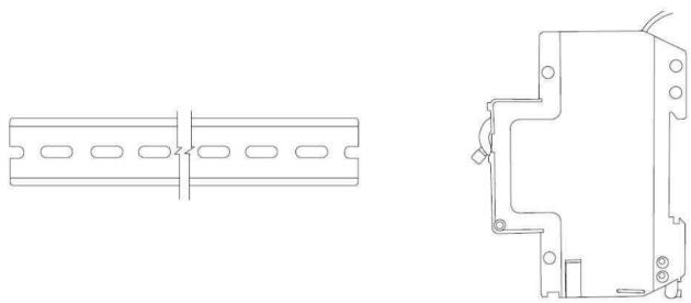
2. Install the product on the rail, and then press the rail clip so that the device on the rail can be fixed in place correctly (When the position is Off).
