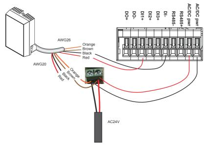
Connect the power inputs from another IR light unit to the same terminal connector.
