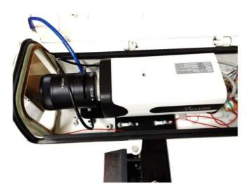
19. Close the top cover of the enclosure, tighten the screws,and secure another screw to the IR bracket.
