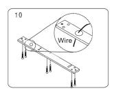
Fix the mounting plate on the door frame according to the holes drilled earlier.
