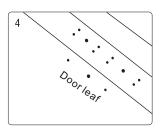
Drill holes based on the marked positions.
