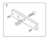
Make a combination based on the picture(add washer accordingly). The rubber ring must be added.
