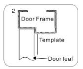
Close the door first, then place the upper side of template on door frame, while adjust the left side next to the door leaf.
