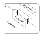
Mark screw positions of armature plate and magnetic lock on door leaf and door frame respectively.
