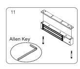
Use Allen key to screw the lock body on the mounting plate.
