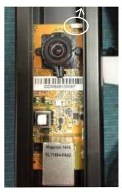
The reset button is used to reset the system or restore the factory default settings. Sometimes resetting the system can return the camera to normal operation. If the system problems remain after a reset, press the reset button longer to restore the factory settings and install again.
