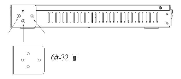
3. Secure the chassis to rack posts using 2 M6 screws on each side.
