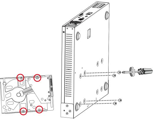
6. Secure the hard disks to the mounting positions in the chassis with its label side facing up, and the connectors facing the inside of the chassis. The sample drawing below shows the positions.
