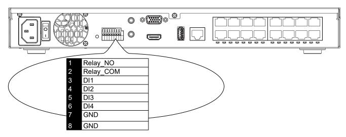
The GND are common ground for the DIs.
