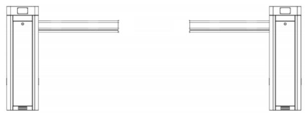
L: Cabinet installed on the left side. The mast goes down to the right side
