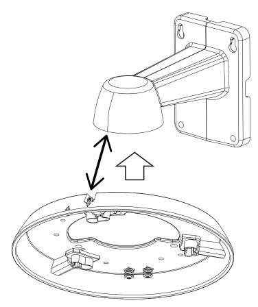
3. When aligned, secure the mounting plate to the AM-21C by driving 3 screws.
