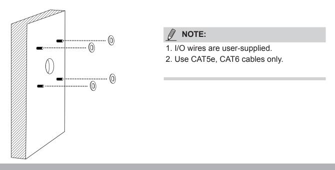
4. Connect power or I/O wires, and use foam tapes or seal foam to ensure the back-end connection is waterproof. The I/O combo cable may be separately purchased.
