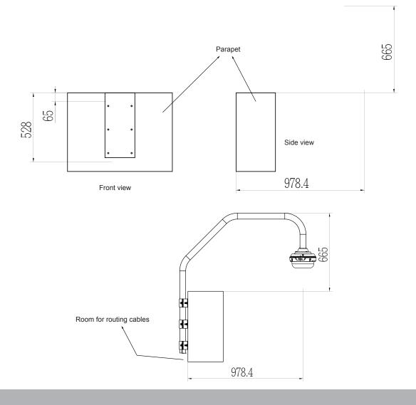
Below is a sample procedure using the parapet mount bracket:
