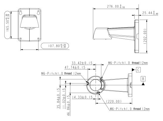
1. The mounting hole definition is illustrated below. The same mounting hole pattern apply to all pole-mount and corner-mount brackets.
