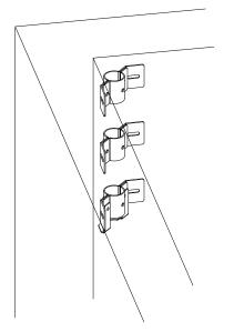
4. Use a crescent wrench to secure the outer brackets to the brackets on the wall using the M8x25 hex bolts and washers. Do not completely tighten the bolts yet! When the speed dome is installed to the mount pipe, it needs to be swiveled out to the desired position.
