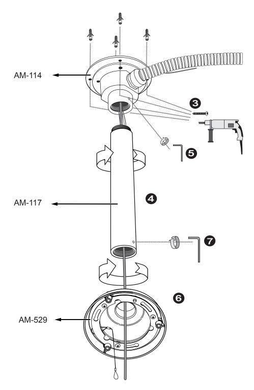
8. Install the camera's top mounting plate to AM-529 by tightening the T25 screws from top.
