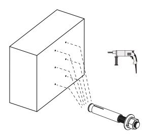
3. Install the brackets to wall using the hex nuts and washers from the sleeve anchors.
