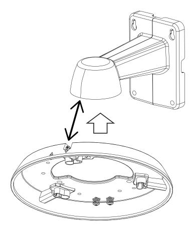
8. When aligned, secure the mounting plate to the AM-21C by driving 3 screws.
