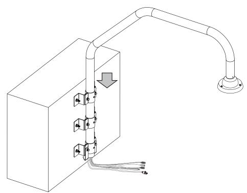
9. Install the camera's top mounting plate to the AM-529. For the rest of the installation details, refer to the documentation that came with the camera.
