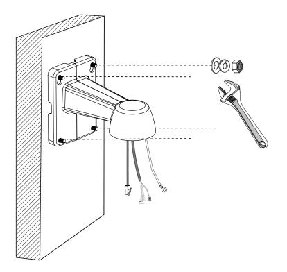
7. Align the top mounting plate with the center of the AM-21C bracket.
