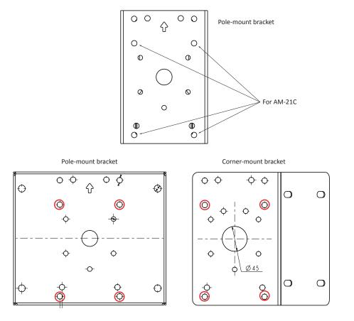
2. Align the top mounting plate with the center of the AM-21C bracket.
