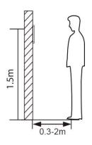
The distance between the device and a user whose height is within 1.4m-1.8m is recommended to be 0.3-2m. Users may slightly move forwards and backwards to improve the quality of facial images captured.
