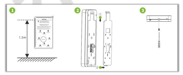
Step 1: Attach the mounting template sticker to the wall, and drill holes according to the mounting paper. Fix the back plate on the wall using wall mounting screws.
