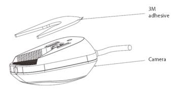
Figure 3-1 Adhesive tape installation
