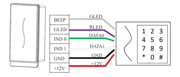
1-Make the connection with the StandAlone equipment at the Wiegand input as shown in the figure.
