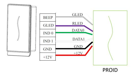
1- Make the connection with the Stand Alone equipment in the wiegand input as shown in the image.
