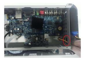
Step 2 Connect the cable into the port.
