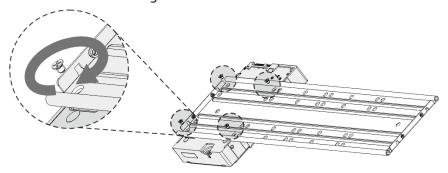
Step 5 Fix other disks on the bracket as needed.
