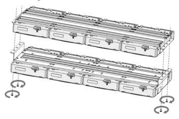
Step 7 Put the drive brackets back and fix them in the DVR.Figure 2-44 Put back drive bracket
