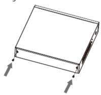
Step 1 Remove the four fixing screws on the rear panel.
