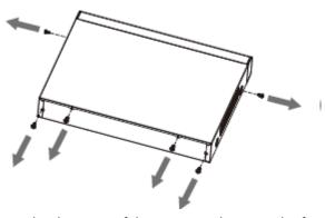
Step 2 Remove the cover in the direction of the arrow as shown in the figure below. Figure 2-15 Remove cover
