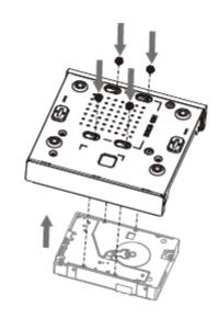
Step 4 Connect HDD to the device using data cable and power cable.
