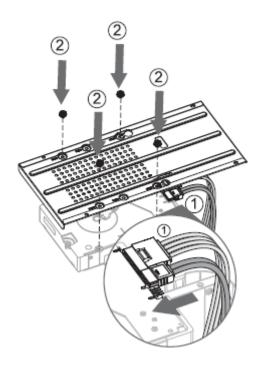
Figure 2-11 Connect cables
