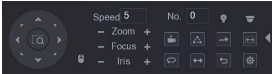
Figure 5-57 Panel de control PTZ ampliado
