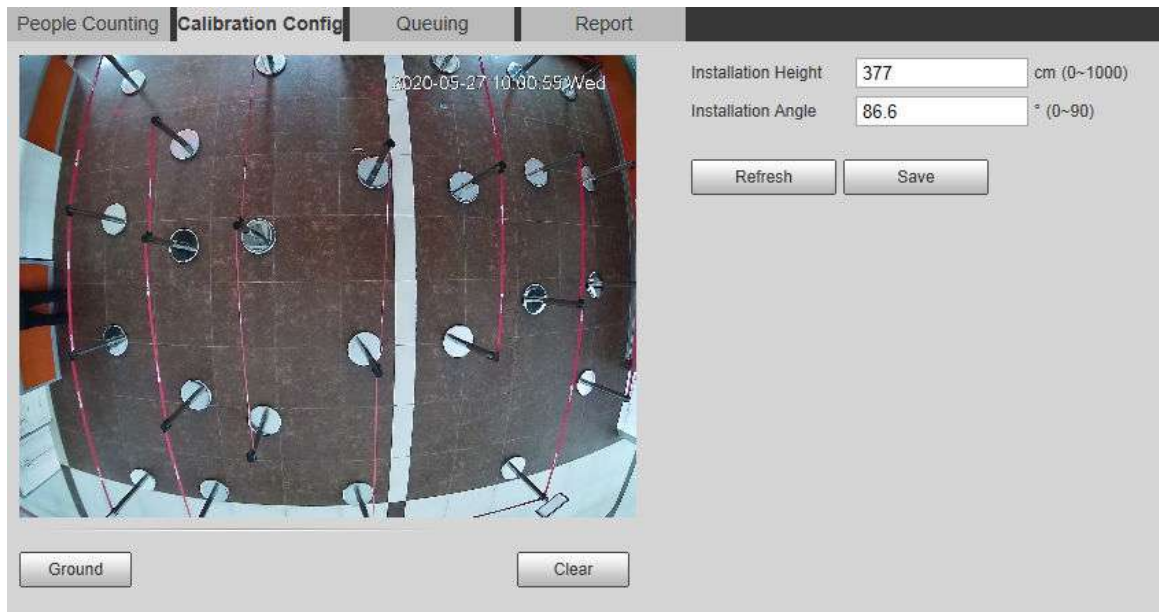
Figure 5-67 Calibration configuration (stereo analysis)
