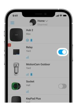
In <u>Ajax apps</u>, you can switch on and off electrical appliances connected to an electrical circuit controlled by Relay Jeweller.
