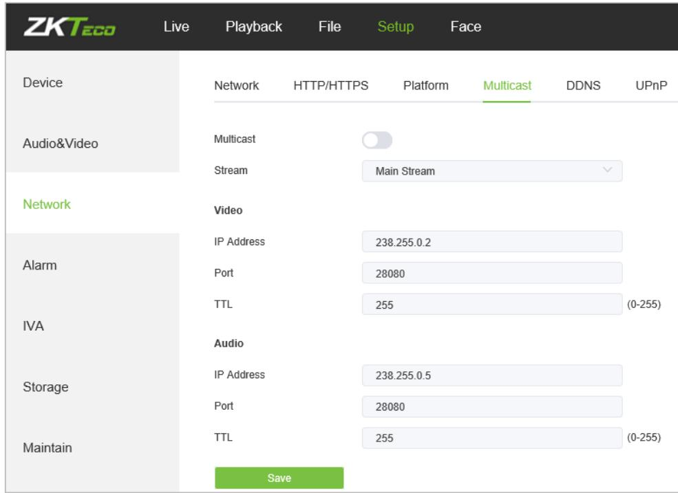
The screenshot shows the 'Multicast' tab selected in the ZKTeco IP camera configuration interface. The 'Multicast' section is enabled, and the 'Main Stream' is selected. Configuration fields include IP Address (238.255.0.2), Port (28080), and TTL (255) for the main stream, and similar fields for sub streams. A 'Save' button is at the bottom.
