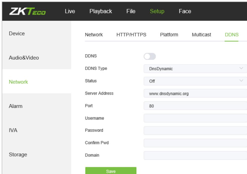
The screenshot shows the 'DDNS' tab selected in the ZKTeco IP camera configuration interface. The 'DDNS' section is enabled, and the 'DnsDynamic' type is selected. Configuration fields include Status (Off), Server Address (www.dnsdynamic.org), Port (80), Username, Password, Confirm Pwd, and Domain. A 'Save' button is at the bottom.
