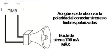
**Figure 1-5 Siren Terminal Wiring**
