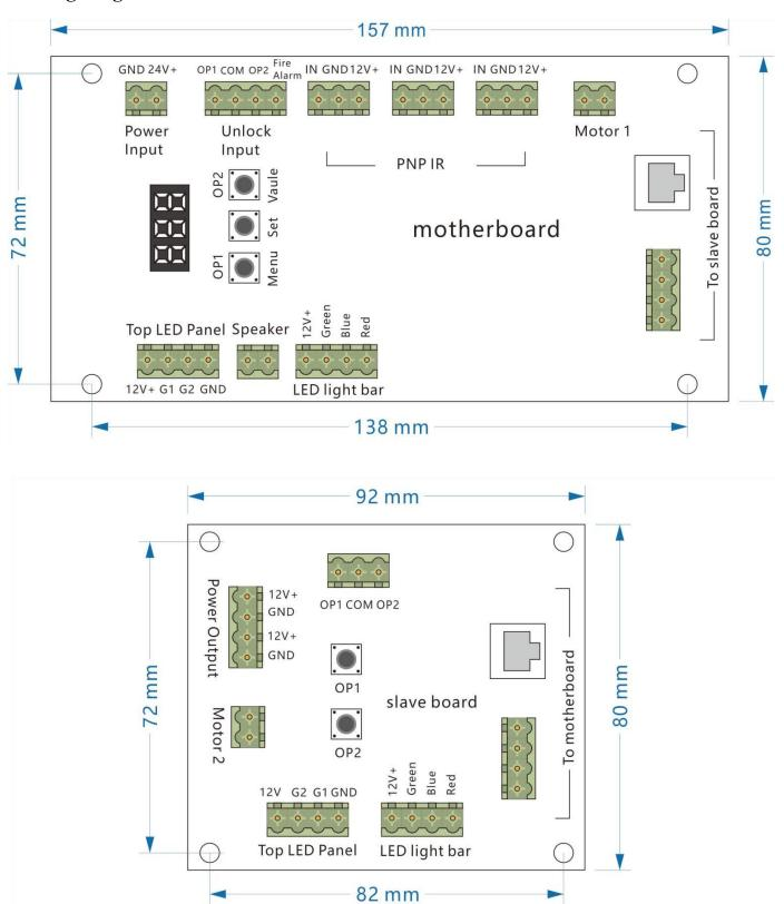
In one channel, there are wires need to be connected between mother board to slave board.
