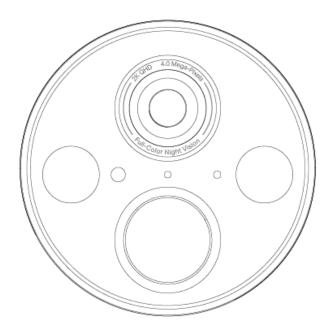
Lens: Located at the top front center for capturing things within its view.
