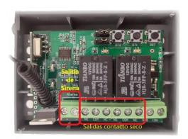
The device configuration offers two usage options for the relay outputs, having the pulse and latching mode;
