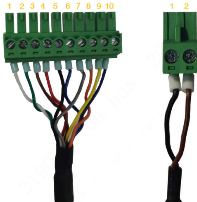
Figure 3-4 Primary antenna and replica antenna terminals (left)/Replica antenna power cable (right)
