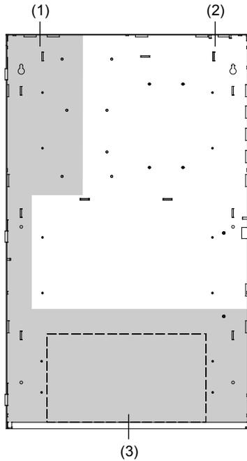
(1) Nonpower-limited wiring area (2) Power-limited wiring area (3) Battery area
