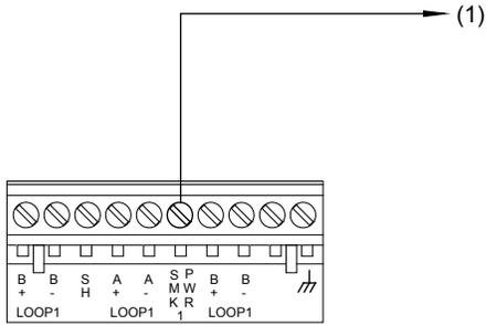
(1) Smoke power to GSA-UM or GSA-MAB for a two-wire smoke detector
