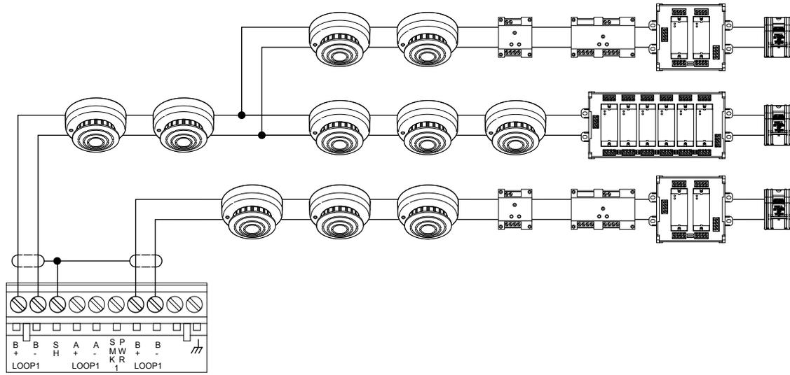
Figure 4: Class A [1] and Class X [2] wiring [1]
