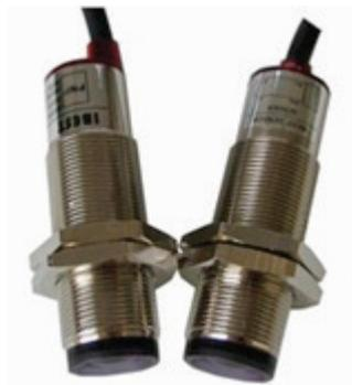
**Cylindrical reflective photoelectric switch:** (the function is the same as above) there are 3 lines in total, including 2 power input, brown + 12V, blue: GND and 1 signal output (black). When a person passes through the reflective photoelectric switch (reflection distance is 10-20mm), the output is + 12V, otherwise it is 0V.
