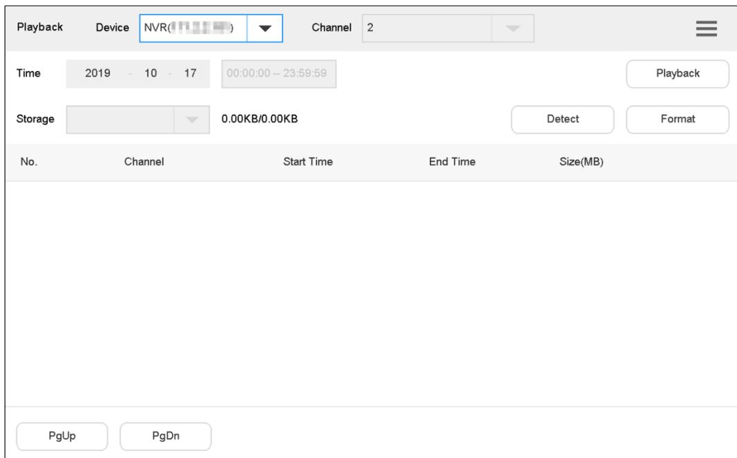
**Step 2** Select playback device and channel, configure time and click **Playback**.
