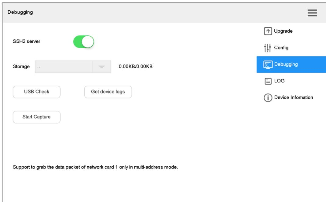
**Step 2** Select **SSH2 server** to enable the **SSH2 server** function.
