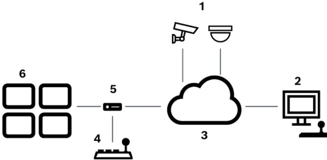
**Figure 5.2:** Scenario 2: Bosch IntuiKey keyboard connected to a decoder
