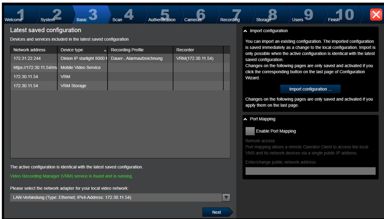
This page displays the latest saved configuration. You can import a BVMS file as a change to the existing configuration. This change is saved but not activated when you click **Next**. You can select the network adapter of your computer that is connected to the video devices (IP cameras, encoders, decoders, iSCSI storage systems) of your system. The IP address of this network adapter is used as IP address of the VRM, the VSG and the local iSCSI storage system.
