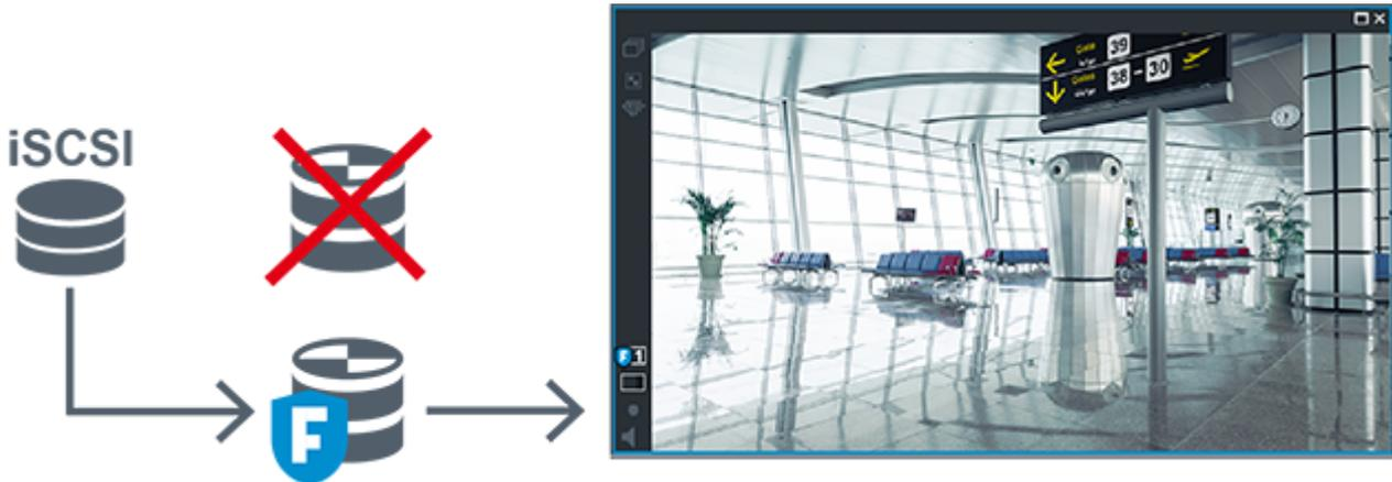
When the Primary VRM and the optional Primary Failover VRM are both not connected, the encoder provides playback. Close the Image pane and display the camera again in an Image pane:
