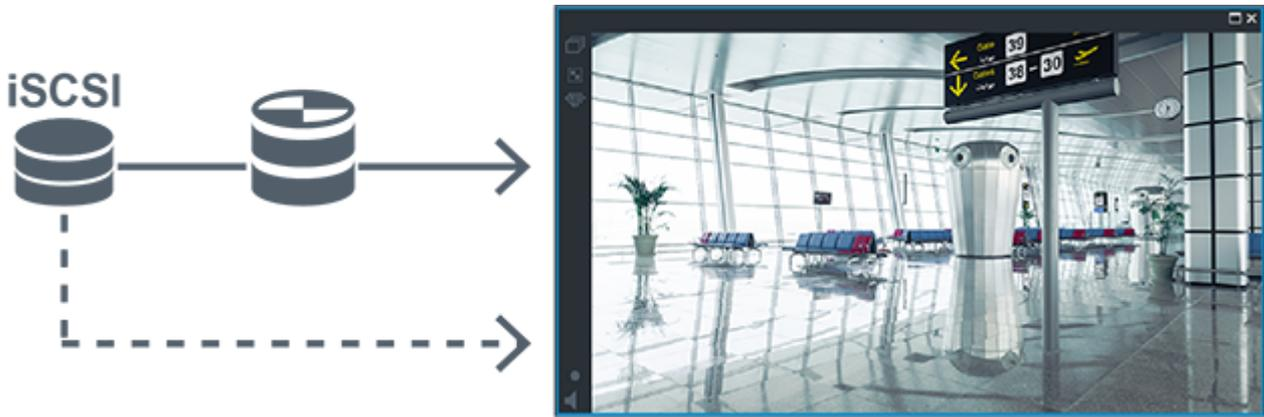
When the Primary VRM is not connected, the configured Failover VRM provides playback. Close the Image pane and display the camera again in an Image pane:
