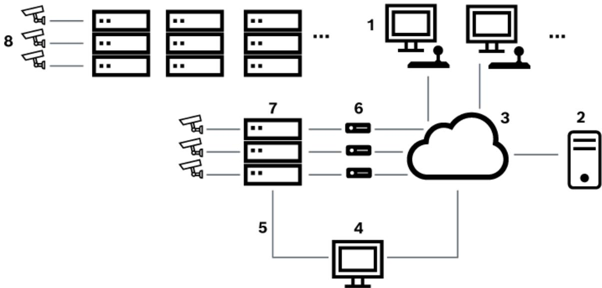
**Figure 5.5:** Bosch Allegiant system extended with Satellite switches
