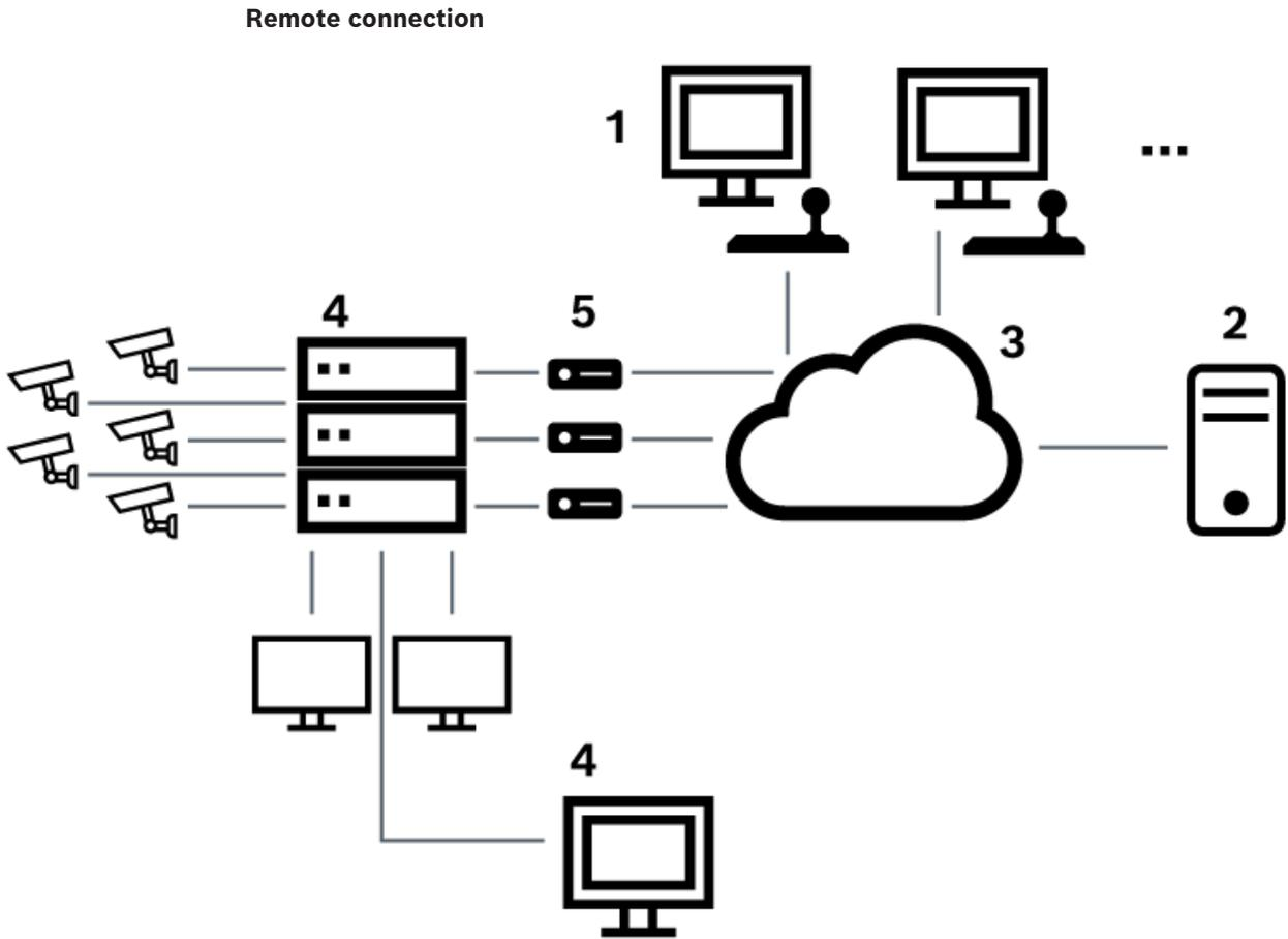
**Figure 5.4:** Bosch Video Management System remote connection to a Bosch Allegiant matrix switch
