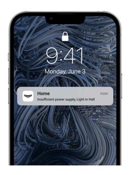
LightSwitch continuously checks its power supply parameters. If LightSwitch controls the power of a lighting appliance with insufficient power (e.g., up to 20 W for LED lighting appliances if a bundled capacitor is not connected), the system will notify users. In this case, it is necessary to replace the lighting
