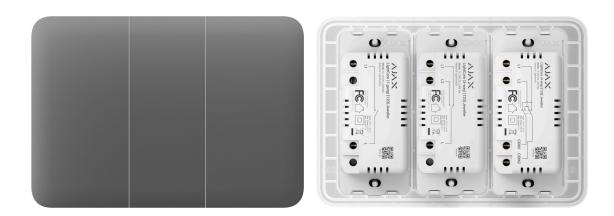
A combined switch consists of several **LightCore** relays and touch-sensitive panels installed into one Frame with the appropriate number of seats.
