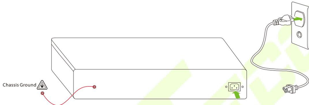
**Note:** Before connecting the power supply, please make sure that the controller is well connected to the chassis ground and the AC ground is truly grounded.
