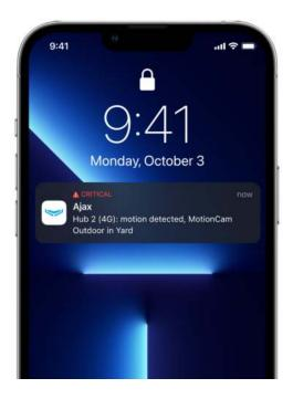
Users know exactly where motion is detected. Notifications contain the name of the hub (name of the protected object), the name of the device and the virtual room to which the detector is assigned.
