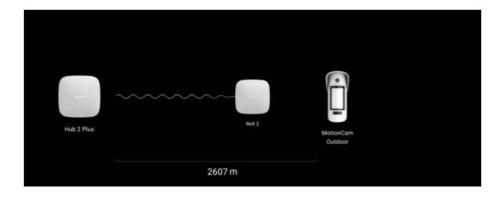
The communication range between ReX 2 and the device is limited by the radio signal range of the device. Radio signal range is indicated on the device page on the website and in the User Manual.
