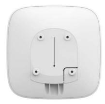
2. Connect ReX 2 to external power supply. Connect an Ethernet cable to ReX 2.
