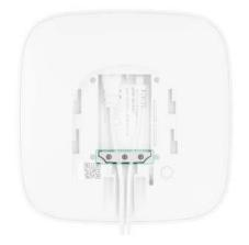
**4.** Slide ReX 2 onto the mounting panel. After installation, check the tamper status in the Ajax app and then the quality of the panel fixation. You will receive a notification if an attempt is made to tear the range extender off the surface or remove it from the mounting panel.
