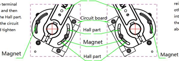
2. If switch left and right, please reinstall the circuit board on the other side and insert the wiring into the other end. Then adjust the magnet according to the above steps.
