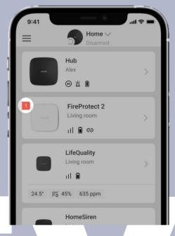
If a FireProtect 2 malfunction is detected (for example, no connection to the hub), the malfunction counter is displayed in the device field in Ajax apps.
