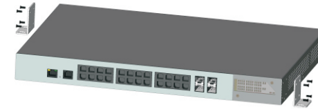
Figure 2-3 Hangers installation diagram
