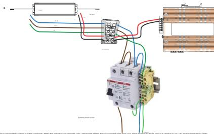
The surge protector wears out after overloads. When the indicator now changes color, replace the shield. You can connect wires from your alarm leminal to the DI pins of a camera so you can receive notification the shield wears out. Check the surge protector, especially after a lightning strike. You can retrieve the related alarm by setting an evert via email, FTP, etc.
