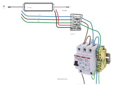
The DC output of the power supply activates a switch PoE as shown below.
