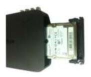
3 Put the HDD into the device.
