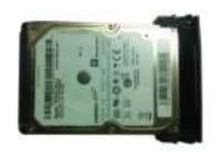
2 Make sure the HDD metal surface is facing up and then put the HDD into the bracket horizontally. After the HDD is in the proper position, the columns on the two sides can lock the screw holes of the HDD to secure
